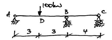
7. For the beam shown, find the reactions and draw the bending moment, shear force, and deflected shape diagrams. Determine the maximum deflection and the rotations at *A*, *B*, and *C*.
