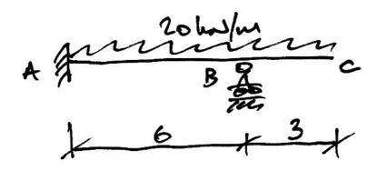
6. For the beam shown, find the reactions and draw the bending moment, shear force, and deflected shape diagrams. Determine the maximum deflection and the rotations at *A*, *B*, and *C*.
