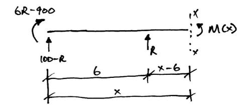
Proceeding as usual, we take moments about the cut, being careful to properly locate the moment reaction at *A* using the correct discontinuity function format:
