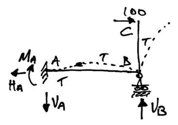
The structure is 1 degree indeterminate. Therefore we need to choose a redundant. Choosing  $V_B$ , we can now calculate the reactions in terms of the redundant by taking moments about A:
