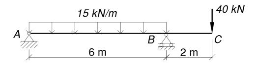
8. (DT004/3 S2R'07) Determine the rotation at A, the rotation at B, and the deflection at C, for the following beam. Check your answer using  $\delta_C = 5wL^4/384EI + PL^3/48EI$ . Take  $E = 200 \text{ kN/mm}^2$  and  $I = 8 \times 10^8 \text{ mm}^4$ . The symbols w, L and P have their usual meanings. (Ans. -360/EI, +360/EI, -697.5/EI)
