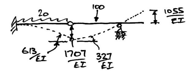
As an aside, we can check our calculation for the deflection at E using the  $S = R\theta$  rule for small displacements. Thus:
