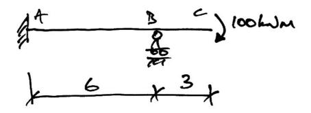
5. For the beam shown, find the reactions and draw the bending moment, shear force, and deflected shape diagrams. Determine the maximum deflection and rotation at *B*.
