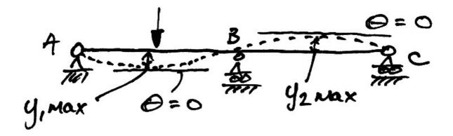
So in this beam we have  $\theta = 0$  at two locations, giving two local maximum deflections,  $y_{1,\text{max}}$  and  $y_{2,\text{max}}$ . The overall largest deflection is  $y_{\text{max}} = \max (y_{1,\text{max}}, y_{2,\text{max}})$ .
