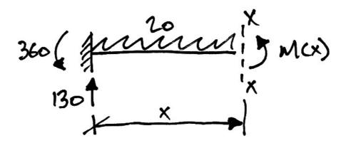
Note that even though it is apparent that there will be tension on the top of the cantilever, we have retained our sign convention by taking M(x) as tension on the bottom. Taking moments about the cut:
