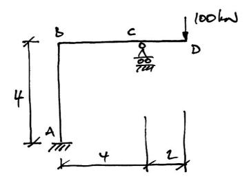
2. For the prismatic frame shown, find the reactions and draw the bending moment, shear force, and deflected shape diagrams. Verify the following displacements:  $\theta_c = 200/EI$ ;  $\delta_{By} = 666.67/EI \downarrow$ ;  $\delta_{Dx} = 400/EI$  (again direction not given because to do so would influence answer).
