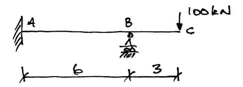
Before starting the problem, consider the qualitative behaviour of the structure so that we have an idea of the reactions' directions and the deflected shape:
