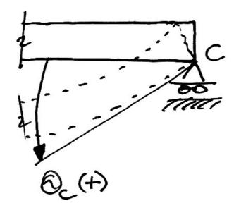
The rotations are thus symmetrical as is expected of a symmetrical beam symmetrically loaded.
