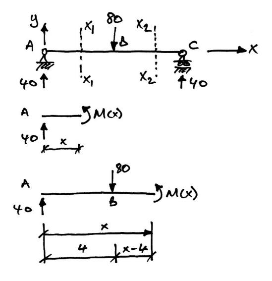
For the free-body diagram A to the cut  $X_1 - X_1$ ,  $\sum M$  about  $X_1 - X_1 = 0$  gives:
