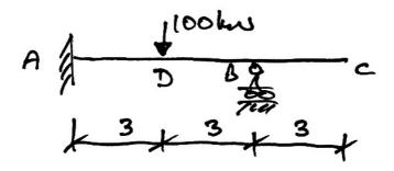
4. For the beam shown, find the reactions and draw the bending moment, shear force, and deflected shape diagrams. Determine the maximum deflection and rotation at *B*.
