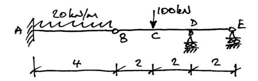
This is a 1 degree indeterminate beam. Once again we must choose a redundant and express all other reactions (and hence displacements) in terms of it. Considering first the expected behaviour of the beam:
