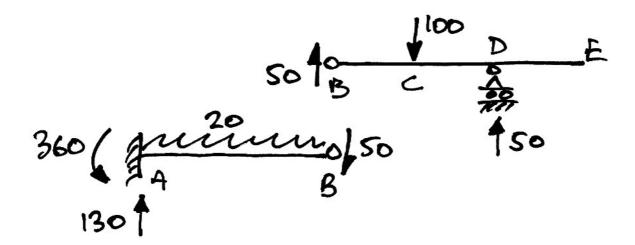
This beam is made of two members: AB and BE. The Euler-Bernoulli deflection equation only applies to individual members, and does not apply to the full beam AB since there is a discontinuity at the hinge, B. The discontinuity occurs in the rotations at B, since the ends of members AB and BE have different slopes as they connect to
