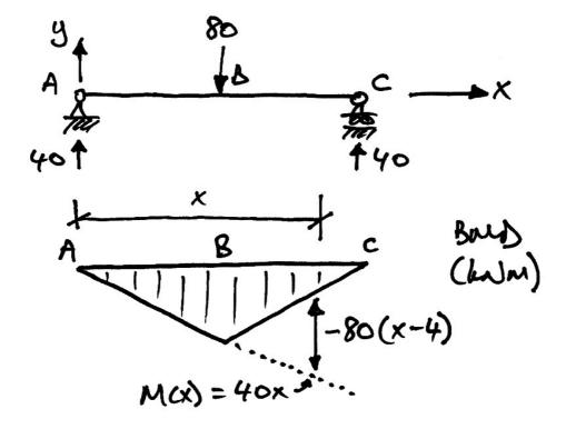
The equations differ by the -80(x-4) term, which only comes into play once we are beyond *B* where the point load of 80 kN is.
