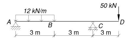
5. (DT004/3 A'05) Verify that the rotation at *A* is smaller than that at *B* for the following beam. Take  $E = 200 \text{ kN/mm}^2$  and  $I = 8 \times 10^8 \text{ mm}^4$ . (Ans.  $\theta_A = -186.67/EI$ ;  $\theta_B = -240/EI$ ;  $\delta_C = -533.35/EI$ ).
